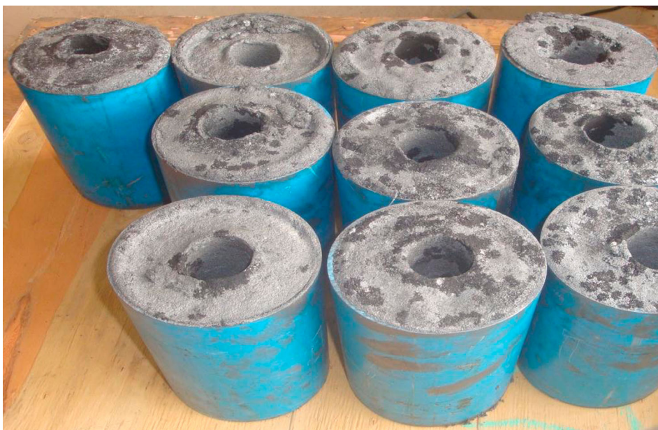
Figure 5. The typical laboratory synthesised rocket composite propellant.
