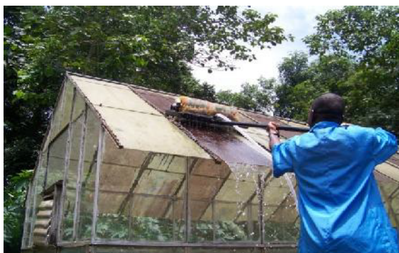
Fig 9. Greenhouse Roof Cleaning using the Designed Cleaner
