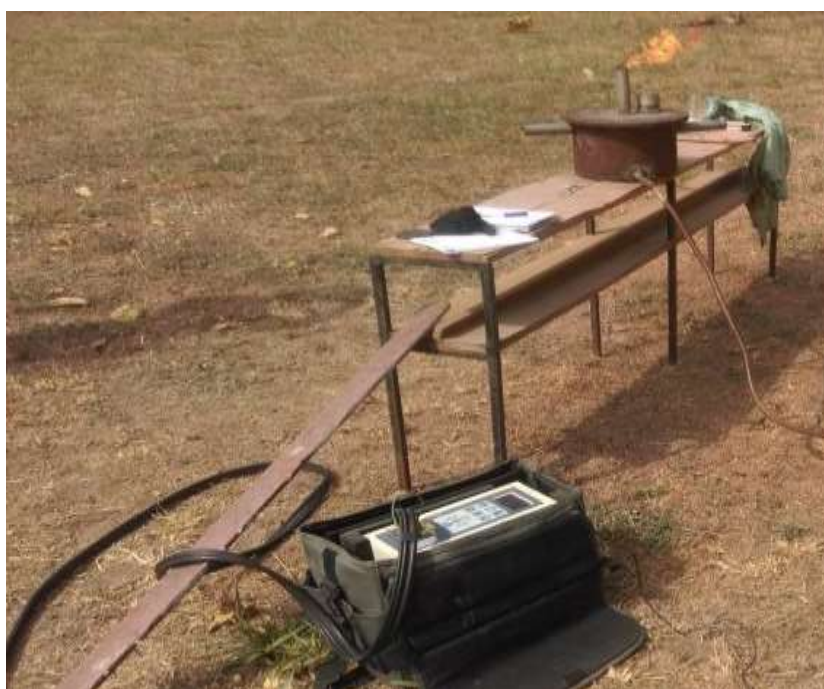
Figure 1: Experimental setup showing the fabricated combustion chamber and the E8500 emission analyser used for pollutant measurement.
