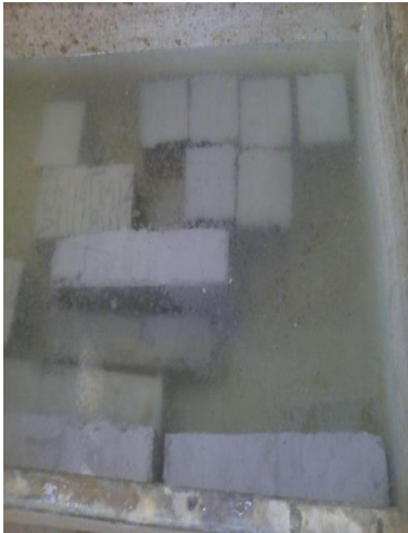
Figure 1: Curing process of beam
