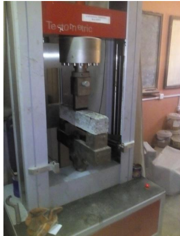
Figure 2: flexural strength test of beam
