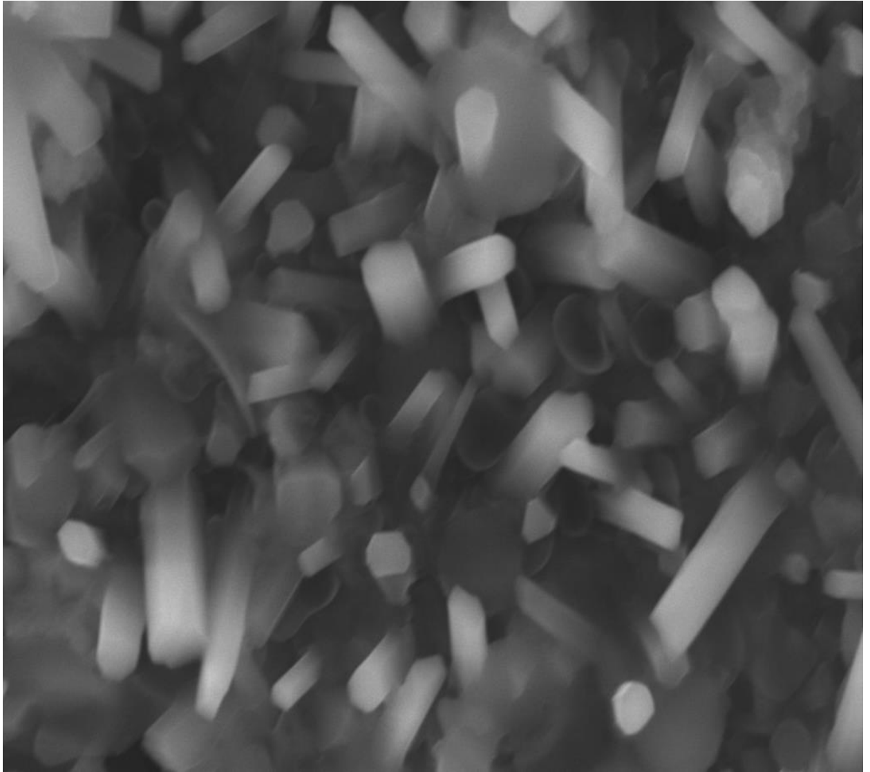
Fig. 4.4b: The scanning electron micrograph (SEM, ZEISS-EVO 18 Research) of nickel ferrite nanorods (NF NR)
