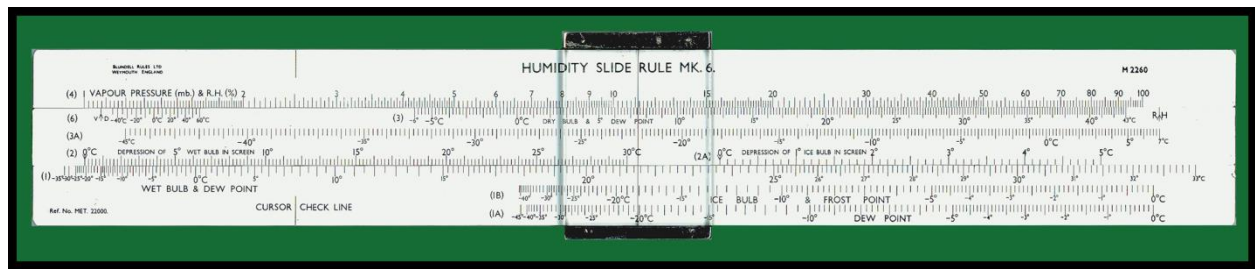
FIGURE 1.1: PHOTOGRAPH OF THE METEOROLOGICAL SLIDE RULE USED IN NIMET STATIONS IN NIGERIA [18]
