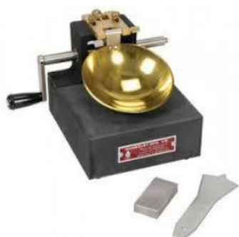
Plate 1: Casagrande Liquid Limit Device
