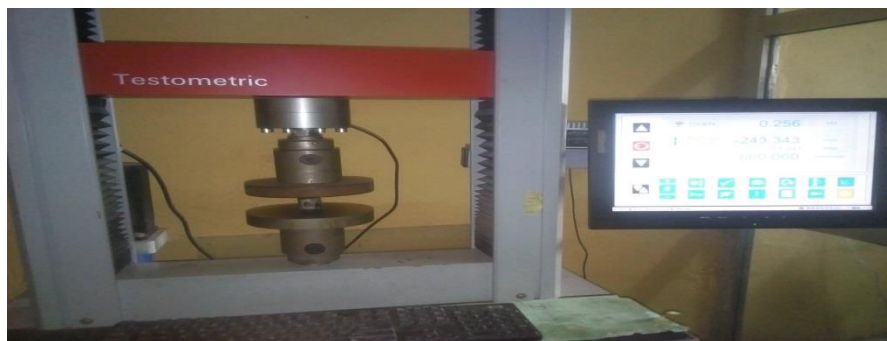
Figure 6: Universal Testing Machine with a clay sample mounted being tested
