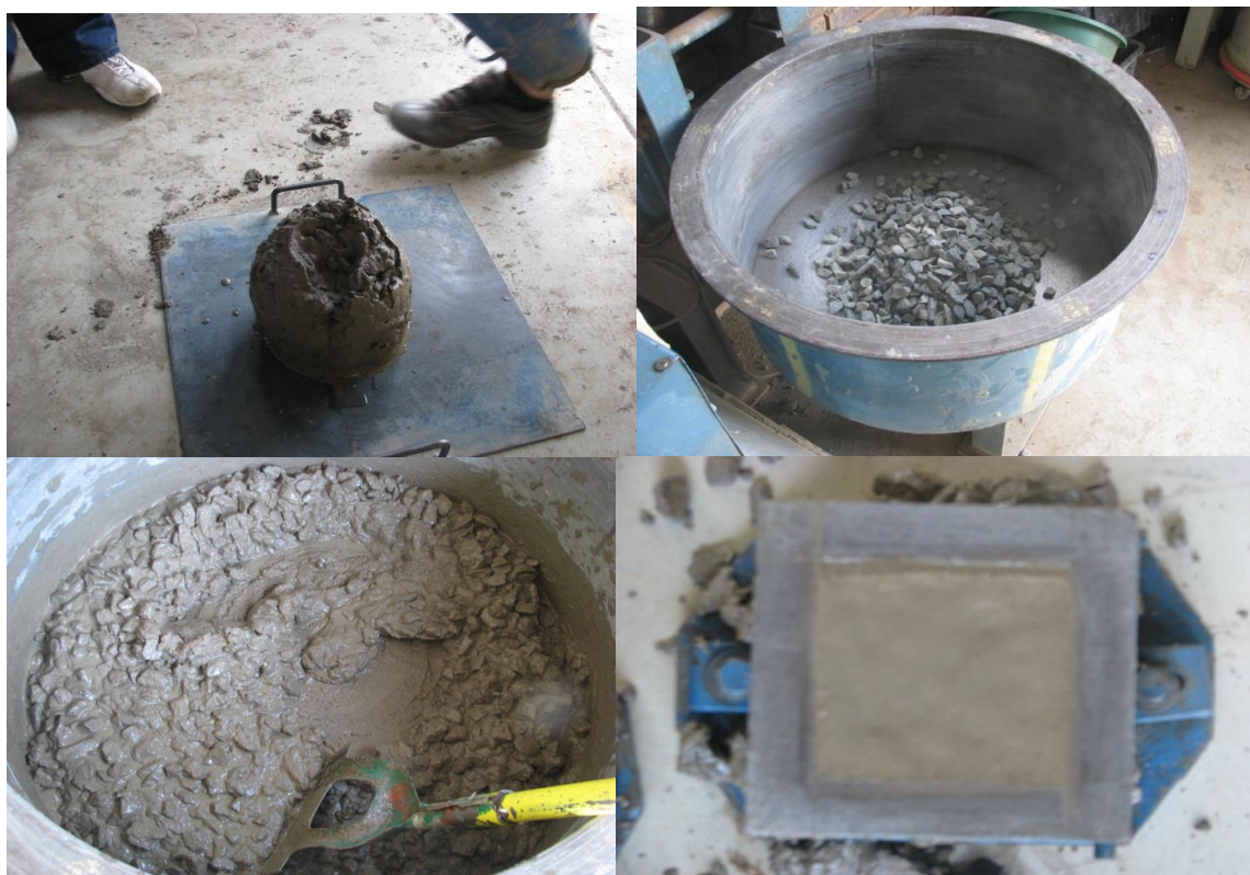
Figure 1: Batching, Mixing and Cast Concrete
