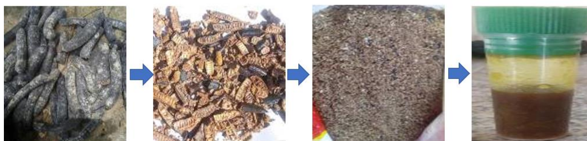
Fig. 1: Prosopis Africana pod oil extraction process
