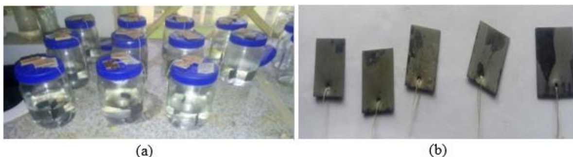
Fig. 2: (a) Weight loss set-up and (b) some of the cleansed specimens after corrosion test
