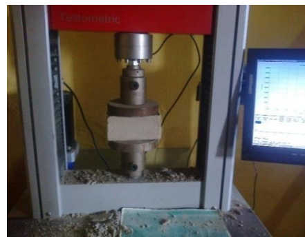
Figure 5: Masonry unit under compressive test
