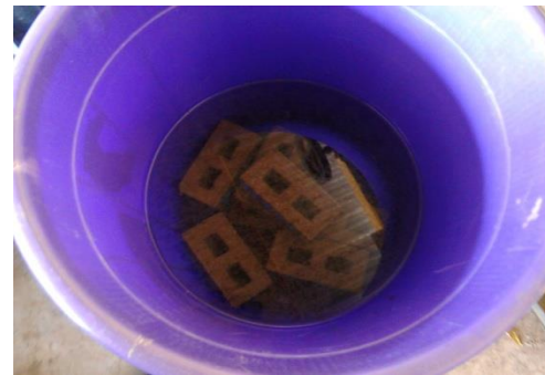
Figure 4: Hollow masonry unit under curing
