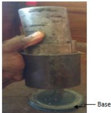
Figure 3 Metal mould used
