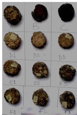
Figure 5 Moulded biomass composites
