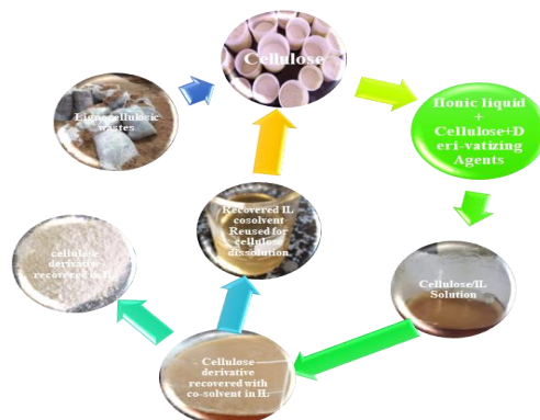
Fig. 5: A description of how to treat cellulosic wastes using an ionic liquid to dissolve cellulose to create fresh material for improved application while also reusing the ionic liquid for another cycle (Baker, 2022).
