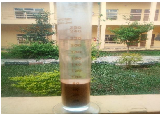
Figure 7: Settled sample after 24 hours
