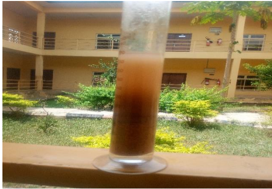
Figure 6: Agitated sample for clay content test
