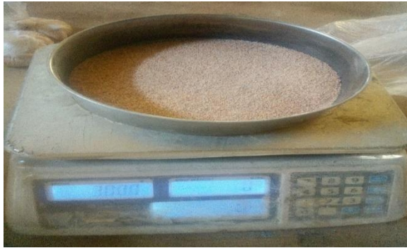
Figure 5: Dry Sample Weighed on the Weighing Balance
