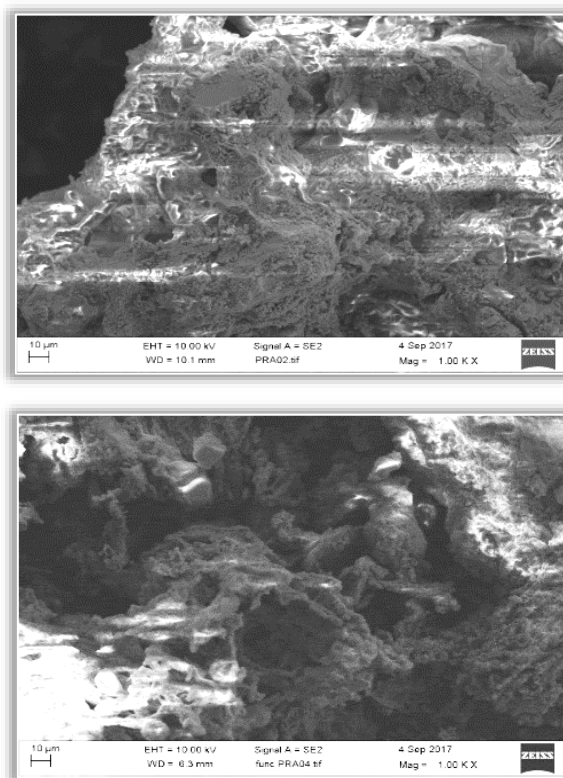
Figure 5: The Morphology of Pyrolysed (Modified) and Functionalised Watermelon Rind.
