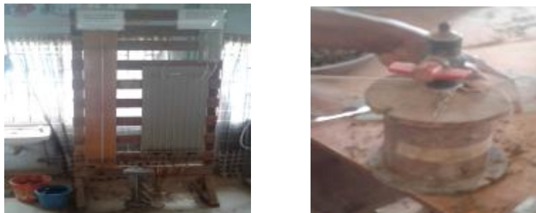
Plate 3: The permeability constant falling head equipment and its mould.
