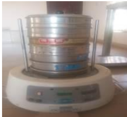
Plate 2: Set of sieve stack on a mechanical sieve shaker used
