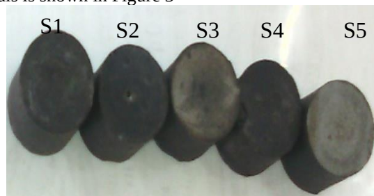
Figure 3: Produced Brake Pad Samples S1, S2, S3, S4 and S5
