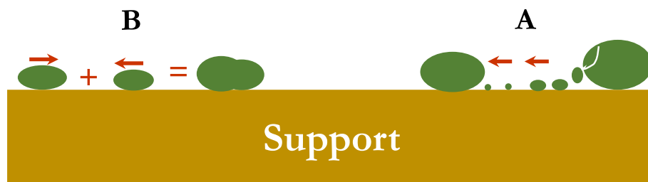
Fig. 6. Pathway to sintering of catalyst via crystal growth by (A) atomic migration, (B) crystallite migration. Modified from Argyle and Bartholomew [165].
